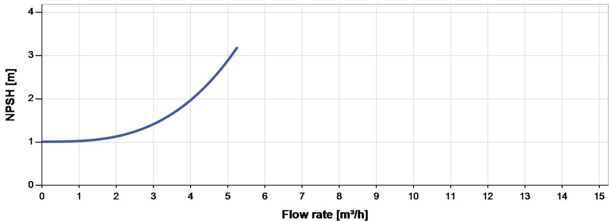
The NPSH (Net Positive Suction Head) is NOT the operating suction head. To calculate the operating suction head please refer to the installation manual.
